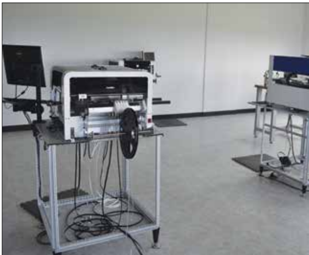
These are the machines that populate the circuit board with its tiny components.
