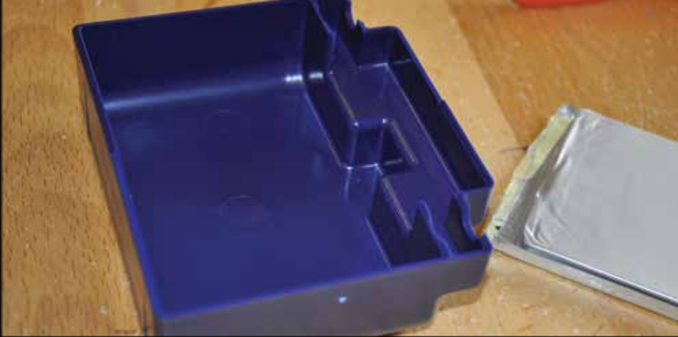
The molded plastic case is designed with a tiny channel around its perimeter, which wicks the liquid glue after assembly.
