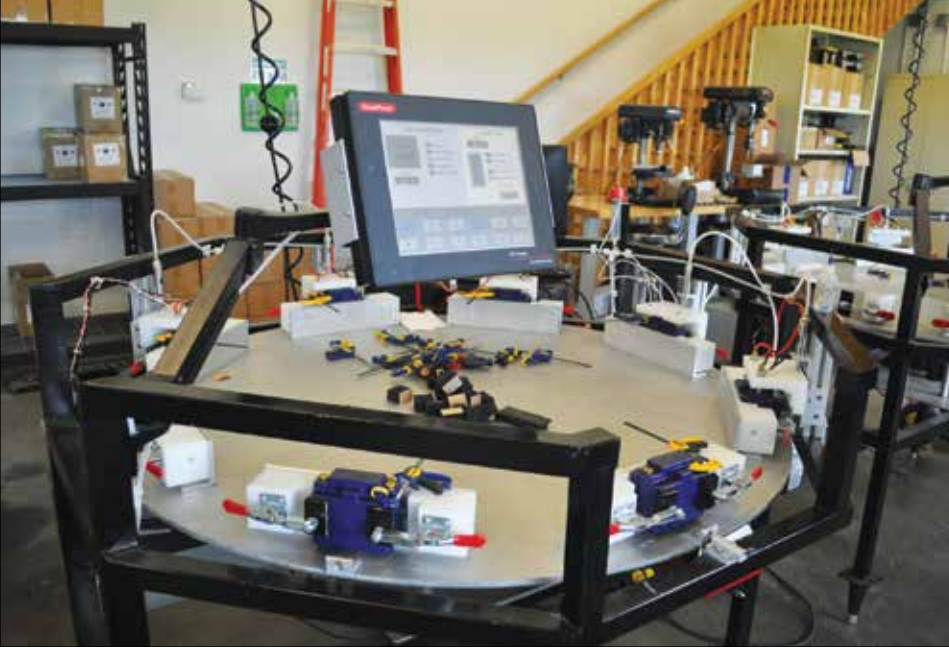
These custom-made assembly and testing tables rotate to expose the battery candidates to a variety of tests and assembly processes.
