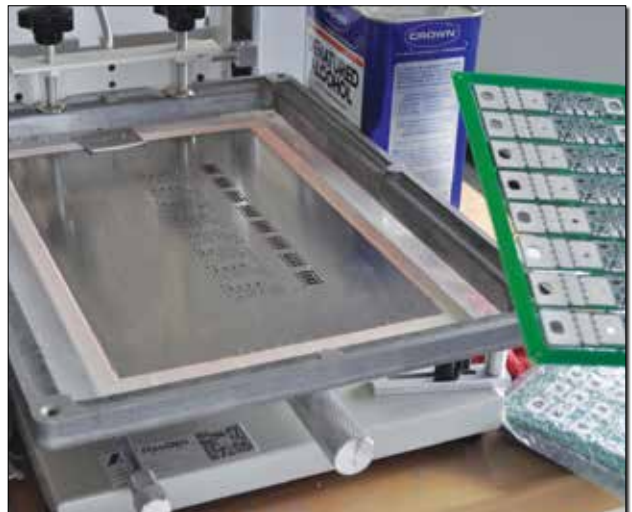
Solder paste is applied to circuit boards in a method similar to silk screening.
