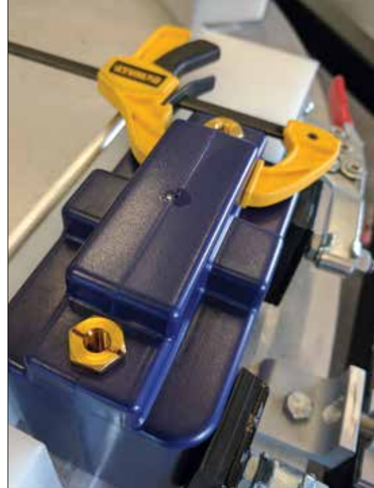
Glue is used to permanently join the clam-shell halves. A small dot of residual glue leaves a shiny spot, which is sometimes mistaken for leakage.
