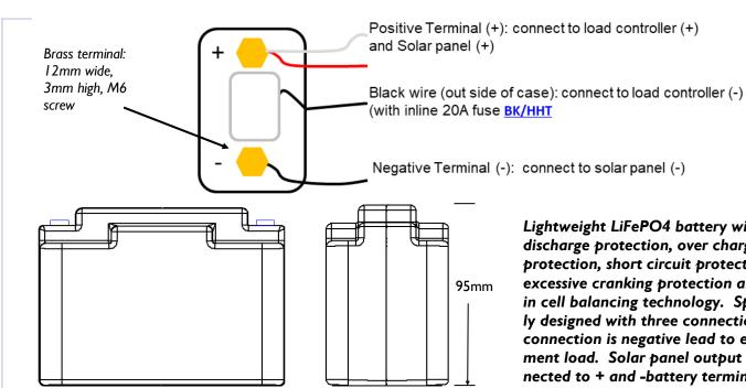
Lightweight LiFePO4 battery with over discharge protection, over charge protection, short circuit protection, excessive cranking protection and built in cell balancing technology. Specifically designed with three connections; third connection is negative lead to equipment load. Solar panel output is connected to + and -battery terminals.
